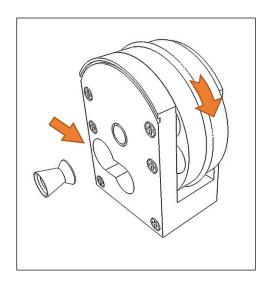
The AZOR AIR RIFLE is designed to use multi-shot magazines. To load the pellets, first we have to extract the magazine drum from the carbine.
