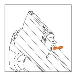
The drum magazine fits into the air rifle housing through a groove and is locked in position by a screw with built-in spring that holds the drum in position.
